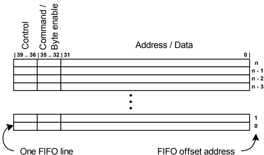
Figure 2.4: Detailed Description of FIFO Register Lines
