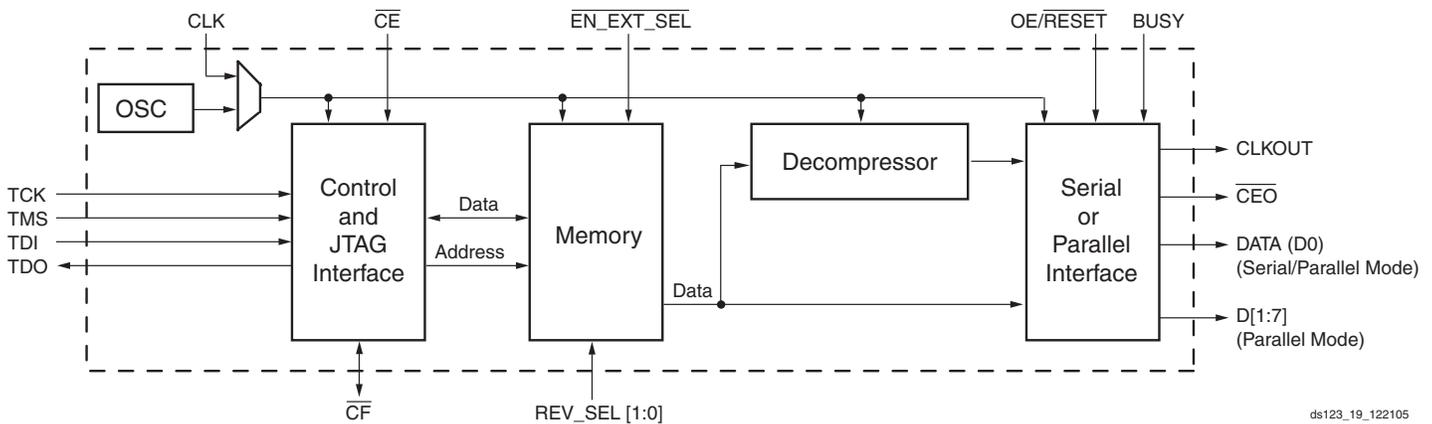
Figure 2: XCFxxP Platform Flash PROM Block Diagram
