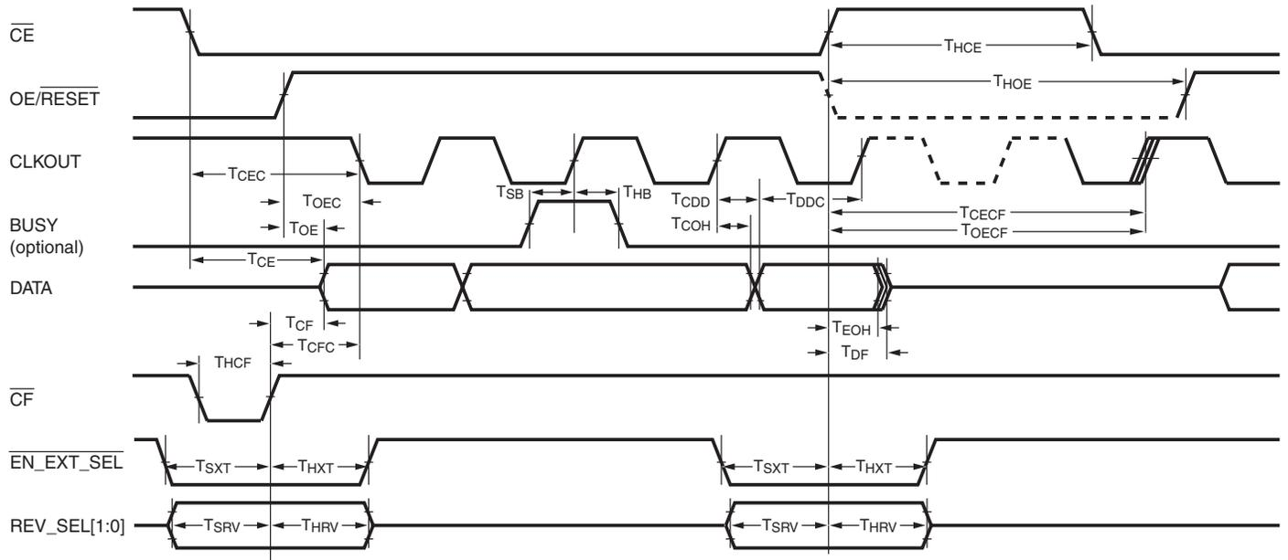
Note: 8 CLKOUT cycles are output after  $\overline{CE}$  rising edge, before CLKOUT tristates, if  $OE/\overline{RESET}$  remains high, and terminal count has not been reached.
