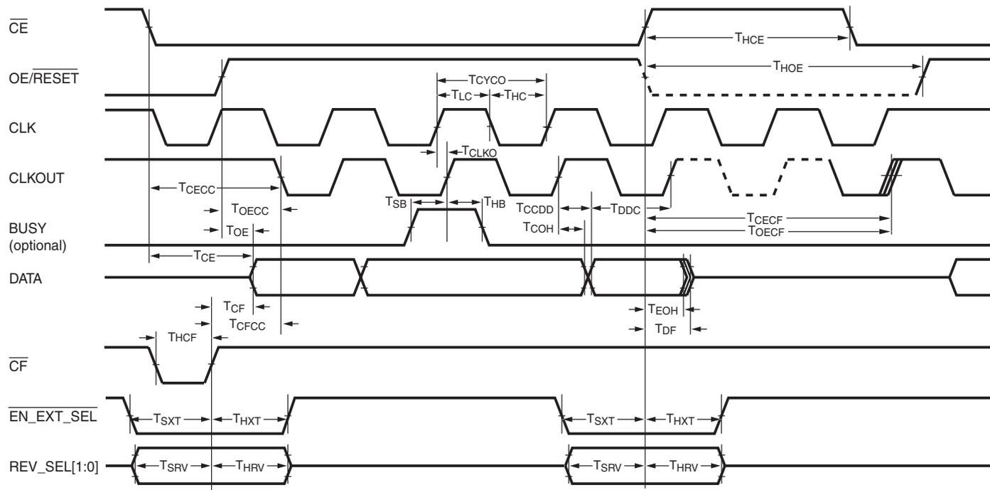
**Note:** 8 CLKOUT cycles are output after  $\overline{CE}$  rising edge, before CLKOUT tristates, if OE/RESET remains high, and terminal count has not been reached.
