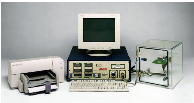
Figure 3-4: \theta_{JA} Measurement Setup
