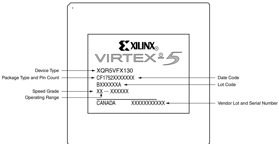
Figure 9-1: Virtex-5QV FPGA Device Package Marking
