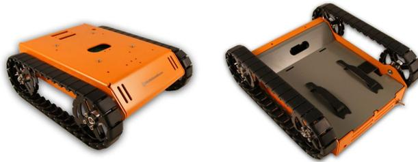
Figure 2.5: The Traxster mechanical kit
