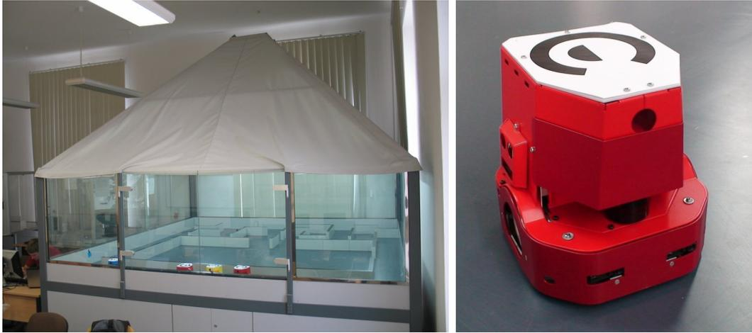
Figure 4.5: SyRoTek arena and robot with dress arc.
