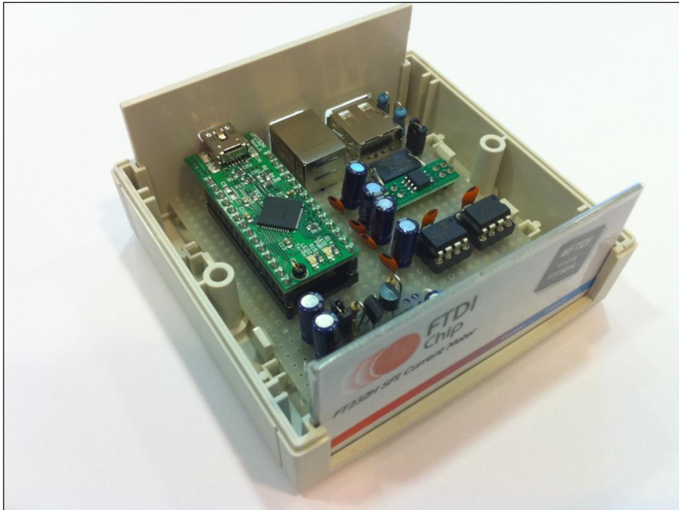
Figure 3 Hardware used for the FT232H USB Current Meter
