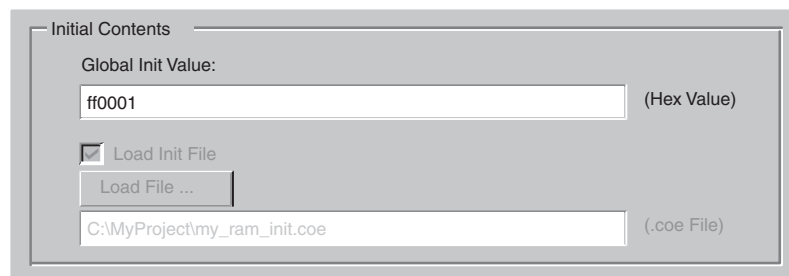
Figure 5-9: Specifying Initial Value for Block RAM Data Output Latches
