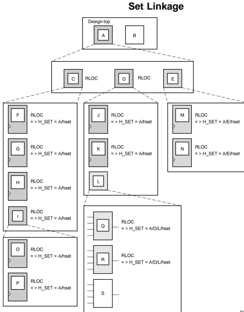
This example shows the process of linking together elements through the design hierarchy. The complete Relative Location specification,  $RLOC=R\ mCn$  or  $RLOC=XmXn$ , is required for a real design.
