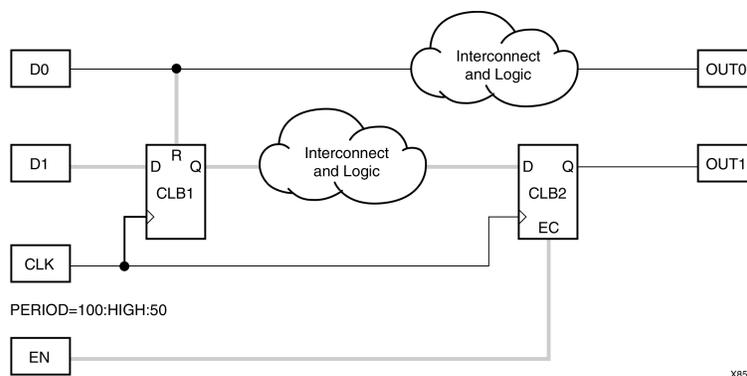
The timing tools do not check pad-to-register paths relative to setup requirements. For example, in the preceding figure, the path from **D1** to Pin **D** of **CLB1** is not included in the Period constraint. The same is true for **CLOCK\_TO\_OUT**.
