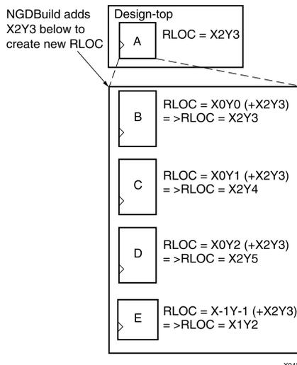
This example illustrates the process of adding RLOC values down the hierarchy. The row and column values between the parentheses show the addition function performed by the mapper. The italicized text prefixed by => is added by MAP during the design resolution process and replaces the original Relative Location constraint that you added.
