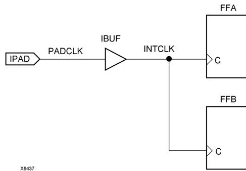
In the preceding design, a Timing Name constraint associated with the **IPAD** symbol includes only the **PAD** symbol as a member in a timing analysis group. For example, the following UCF file entry creates a time group that includes the **IPAD** symbol only.
