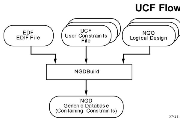
UCF files are input to NGDBuild (see the preceding figure). The constraints in the UCF files become part of the information in the NGD file produced by NGDBuild. For FPGA devices, some of these constraints are used when the design is mapped by MAP, and some of the constraints are written into the Physical Constraints File (PCF) produced by MAP.
