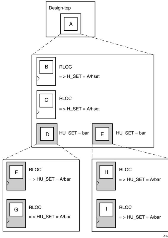
This example shows how HU SET constraints link elements in the same node together by naming them with the same identifier. Because of the same name (*bar*) on two elements, D and E, the elements tagged with Relative Location constraints below D and E become part of the same HU SET.
