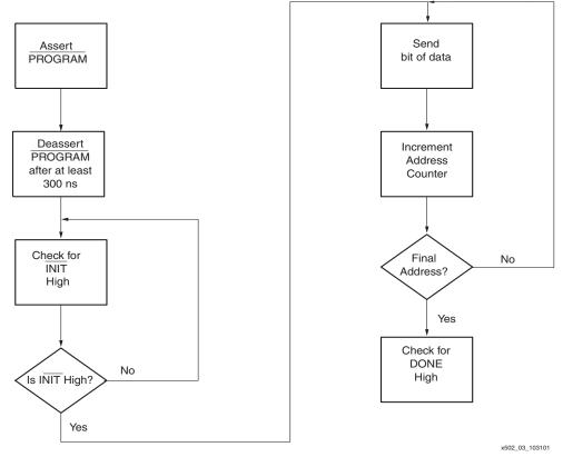
Figure 11: Slave Serial Configuration Flow Diagram
