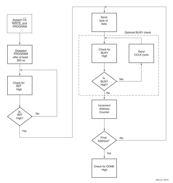
Figure 8: Select MAP Configuration Flow Diagram
