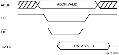
Figure 13: Read-Cycle Timing Diagram
