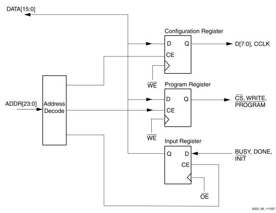
Figure 7: CPLD Block Diagram
