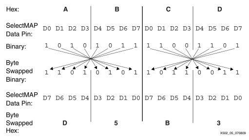
Figure 3: Byte-Swapping Example
