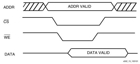
Figure 12: Write-Cycle Timing Diagram
