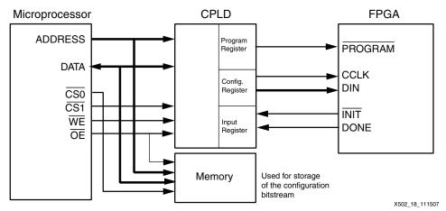
Figure 9: Slave Serial Configuration
