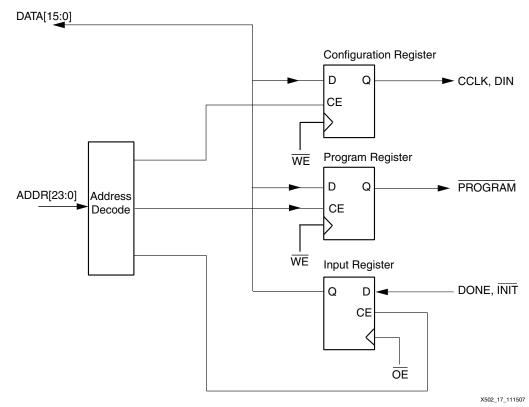
Figure 10: CPLD Block Diagram
