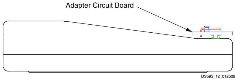
Figure 12: Flying Wire Adapter (Side) without Wires
