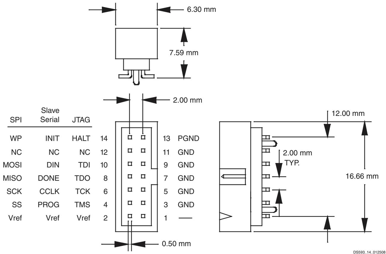
Figure 14: Target Interface Connector Dimensions and Signal Assignments
