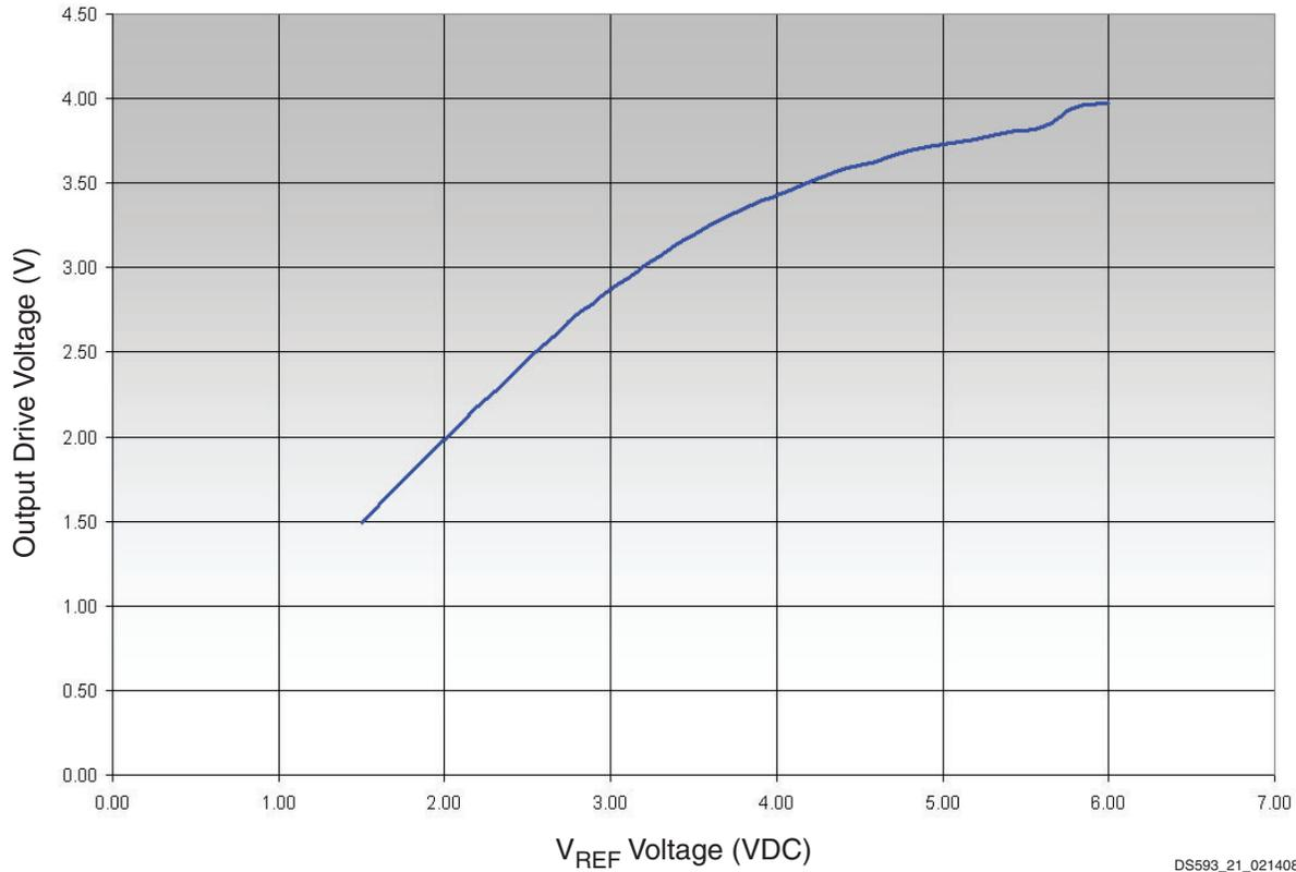
Figure 21: Output Drive Voltage vs. V<sub>REF</sub>
