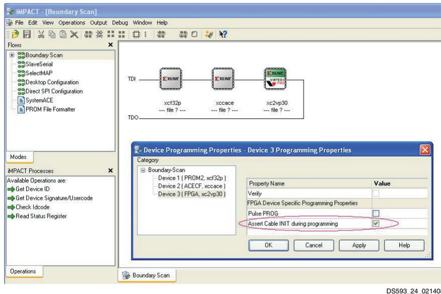
Figure 24: Enabling the HALT Signal in iMPACT (9.2i)
