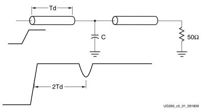
Figure 5-1: TDR Signature of Shunt Capacitance
