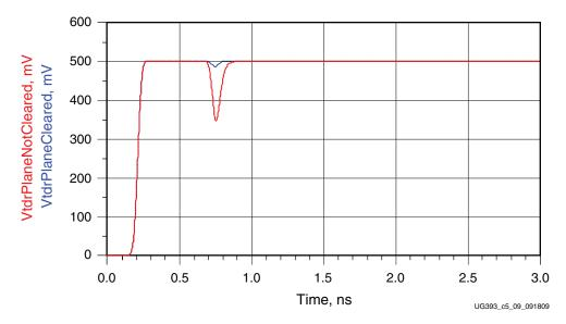
Figure 5-9: TDR Results Comparing 0402 Pad Structures
