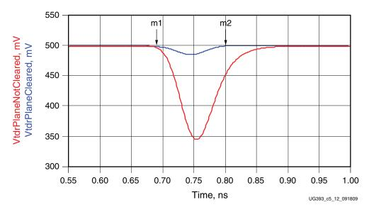
Figure 5-12: 57 fF Excess Capacitance with Ground Plane Intact
