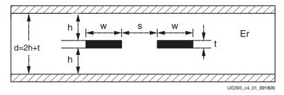
Figure 4-1: Differential Edge-Coupled Centered Stripline
