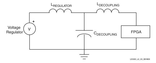
Figure 2-3: Simplified PDS Circuit
