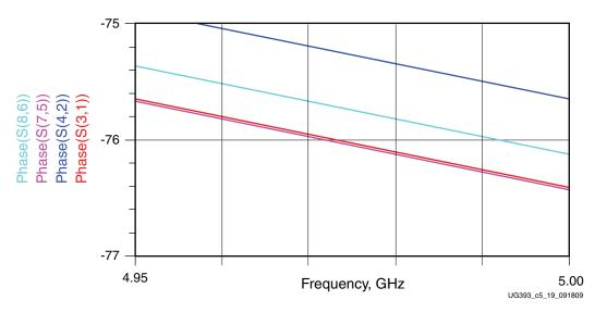
Figure 5-19: Simulated Phase Response of 45 Degree Bends with Jog-Outs
