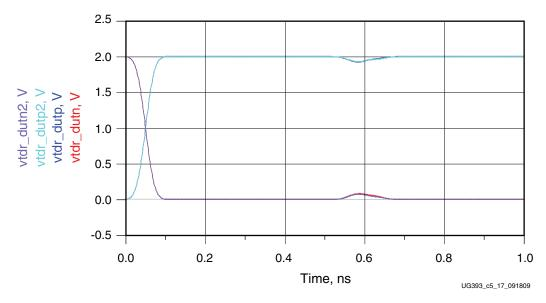
Figure 5-17: Simulated TDR of 45 Degree Bends with Jog-Outs
