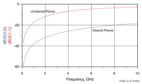
Figure 5-7: Return Loss Comparison Between 0402 Pad Structures
