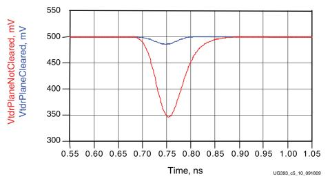
Figure 5-10: TDR Results Comparing 0402 Pad Structures
