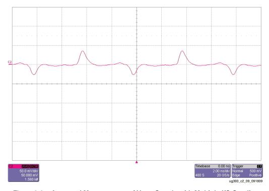
Figure 2-9: Averaged Measurement of V<sub>CCO</sub> Supply with Multiple I/O Sending Patterns at 250 Mb/s
