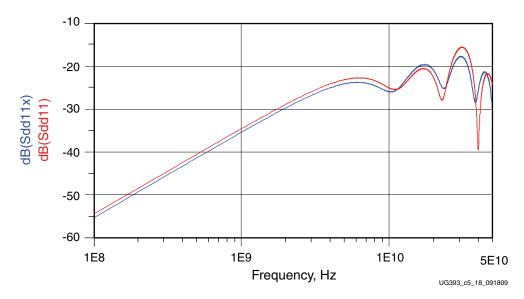
Figure 5-18: Simulated TDR of 45 Degree Bends with Jog-Outs
