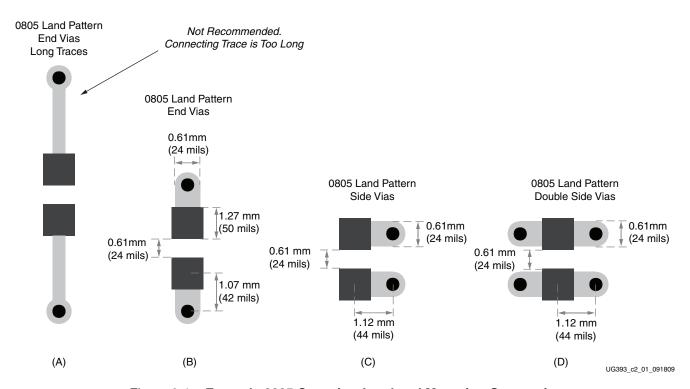
Figure 2-1: Example 0805 Capacitor Land and Mounting Geometries
