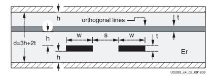
Figure 4-2: Differential Edge-Coupled Offset Stripline
