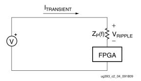
Figure 2-4: Further Simplified PDS Circuit
