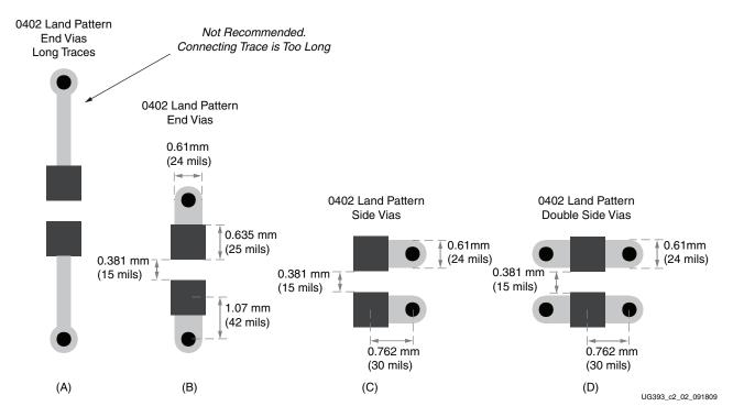
Figure 2-2: Example 0402 Capacitor Land and Mounting Geometries
