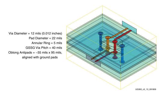
Figure 5-13: Differential Via Design Example
