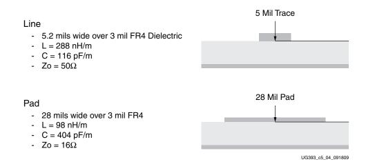
Figure 5-4: 2D Field-Solver Analysis of 5 Mil Trace and 28 Mil Pad
