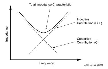
Figure 2-6: Contribution of Parasitics to Total Impedance Characteristics
