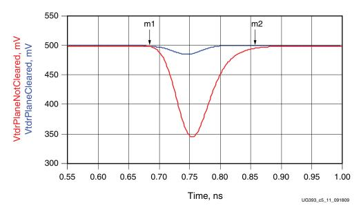
Figure 5-11: 840 fF Excess Capacitance with Ground Plane Intact
