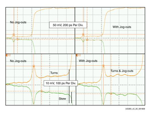
Figure 5-20: Measured TDR of 45 Degree Bends with and without Jog-Outs
