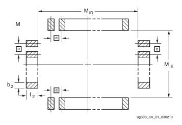
Figure A-1: EIA Standard Board Layout of Soldered Pads for QFP Packages
