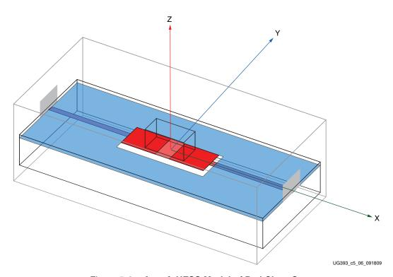
Figure 5-6: Ansoft HFSS Model of Pad Clear-Out
