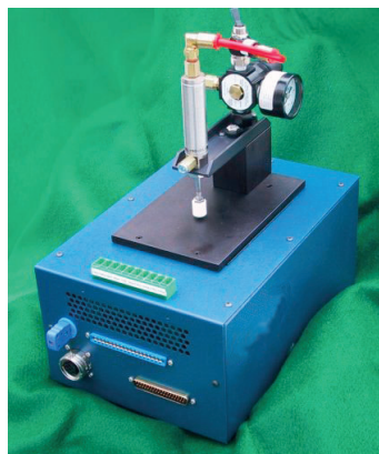
Figure 3-9: \theta_{JC} Measurement Setup
