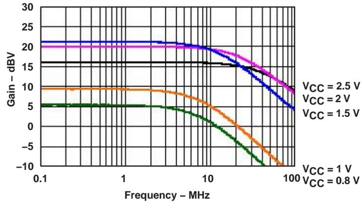
**Figure 6. Open-Loop Gain Characteristics of AUC1GU04**
