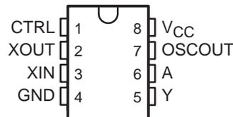
Figure 16. Pinout Diagram for LVC1404
