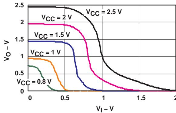
Figure 9.  $V_O$  vs  $V_I$  Characteristics of AUC1GU04
