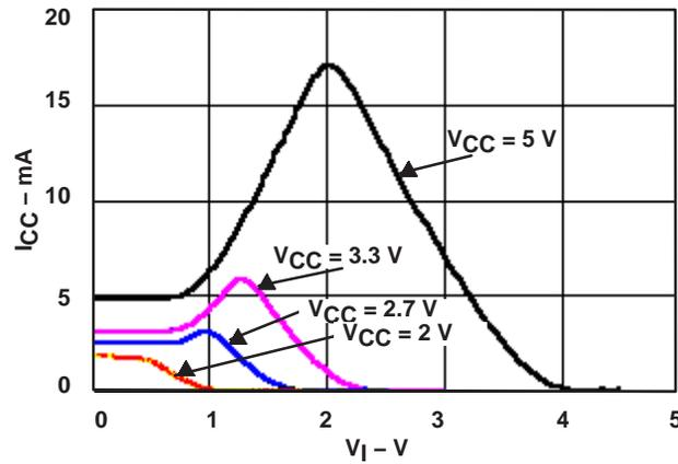
Figure 11.  $I_{CC}$  vs  $V_I$  Characteristics of AHC1GU04
