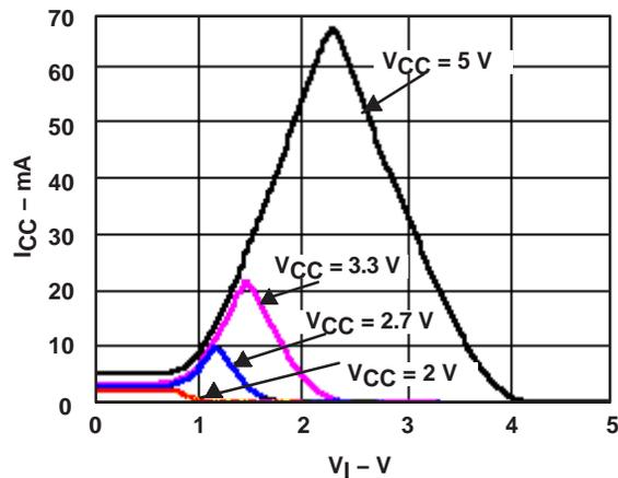
Figure 10.  $I_{CC}$  vs  $V_I$  Characteristics of LVC1GU04
