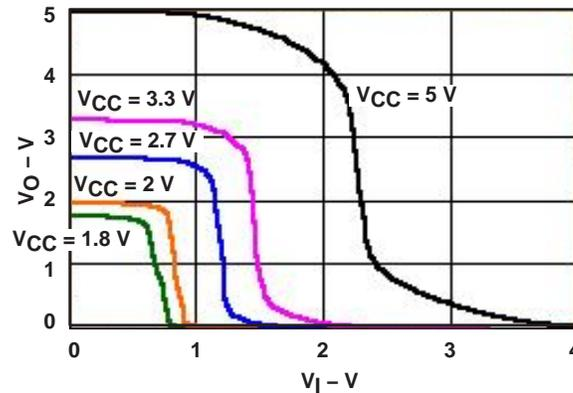
**Figure 7.  $V_O$  vs  $V_I$  Characteristics of LVC1GU04**
