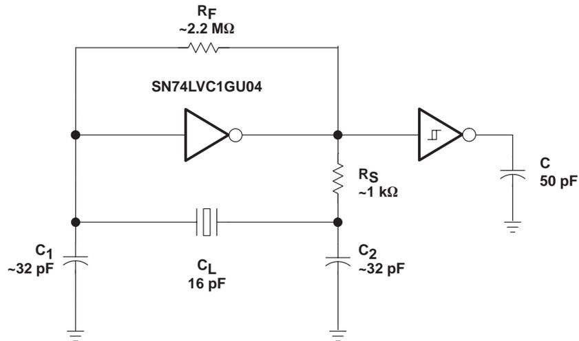
**Figure 24. Oscillator Circuit Using a Schmitt-Trigger Input Inverter**
