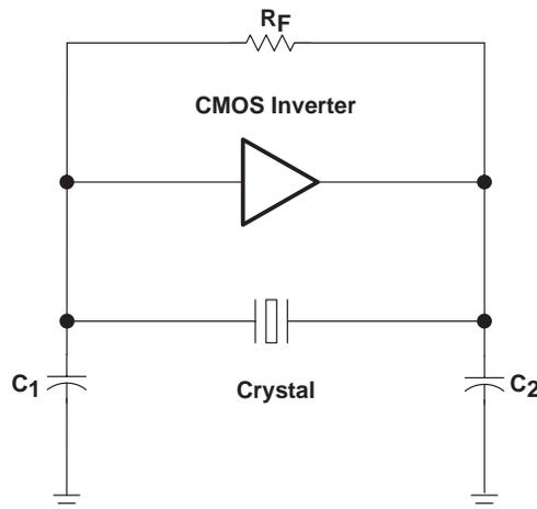
**Figure 3. Pierce Oscillator Using CMOS Inverter**
