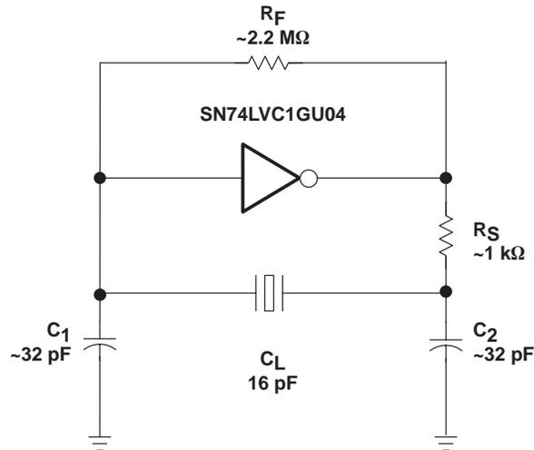
Figure 19. Pierce Oscillator Circuit Using Unbuffered CMOS Inverter
