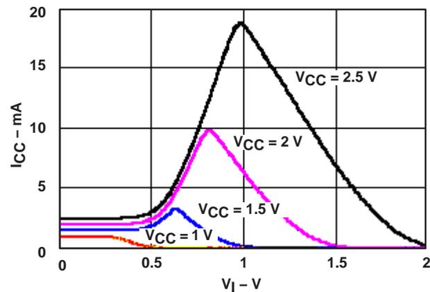
Figure 12.  $I_{CC}$  vs  $V_I$  Characteristics of AUC1GU04
