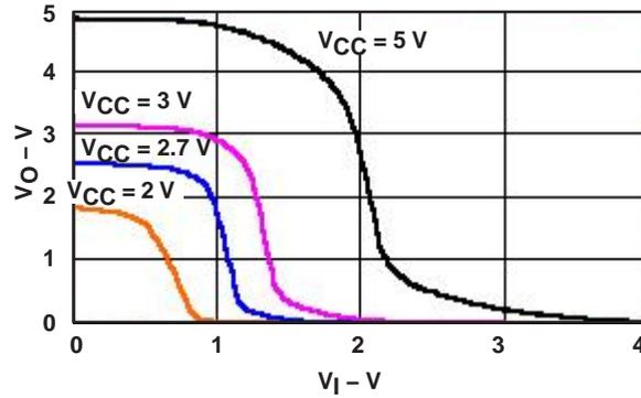
Figure 8.  $V_O$  vs  $V_I$  Characteristics of AHC1GU04
