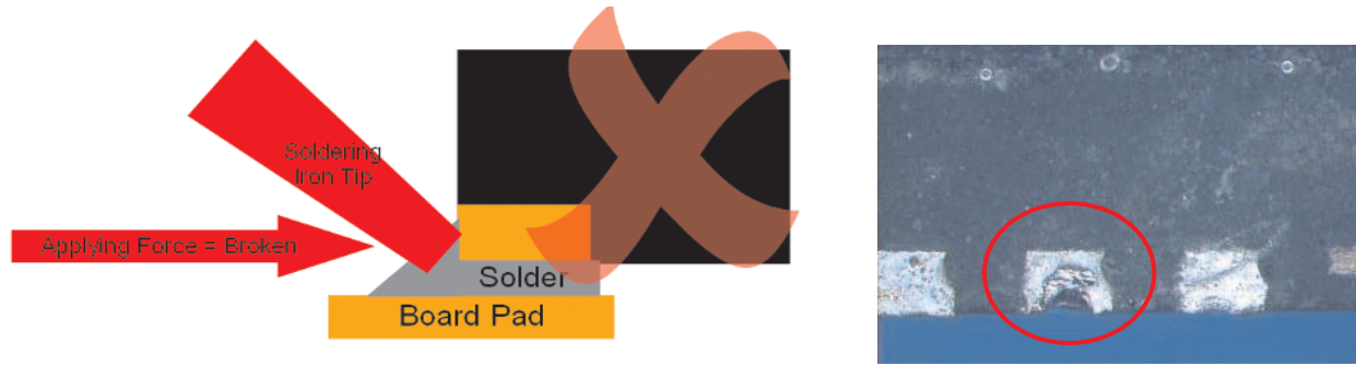
Figure 18. Manual Rework Damage
