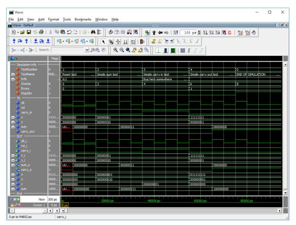
During a simulation, the waveform window shows current test number, test name, user-defined info, accumulated number of checks and errors. When the error counter increments, a bug has been found in that point in time.
