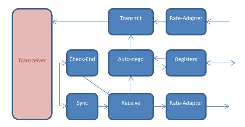
Sync block: which sync into the received character and gives odd/even flag and type of the received order-set. The first code-group of any ordered set must be "even".
