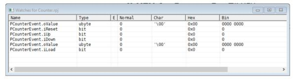
Now keep using the *Control Panel* to send events and observe the results in the watch windows. You will not see the events since their duration is only one step and the RVM is running continuously.
