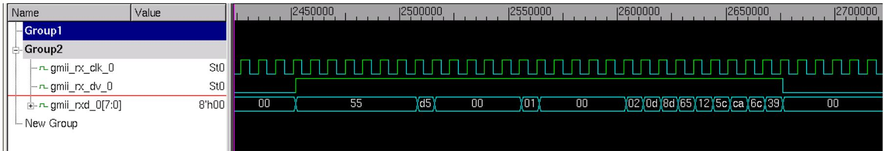
The above waveform shows a sample packet reception. RX\_DV is asserted for the entire time the packet is transmitted, and the low to high transition on RX\_DV indicates start of transmission.
