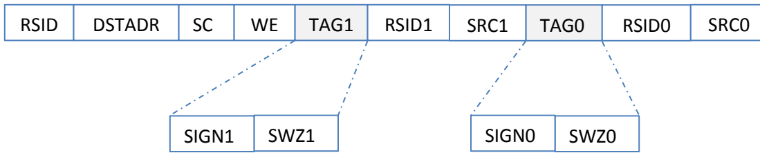
Figure 40 The decoded instruction presented by the IIU to the SMU
