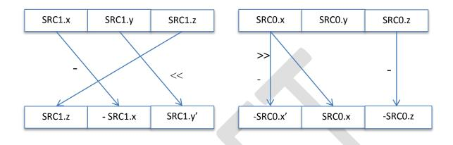
Figure 23 Combining several source modifiers in a single instruction
