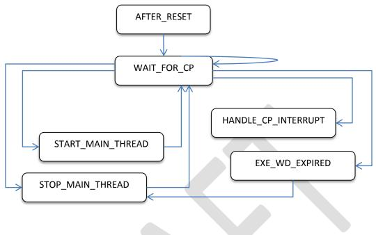
Figure 12 Control FSM
