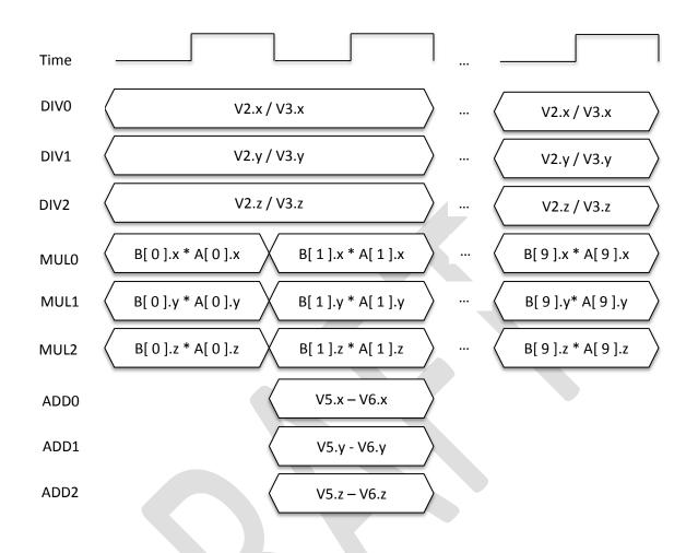
Figure 14 Behaviour of the execution units over time for the example from Figure 13
