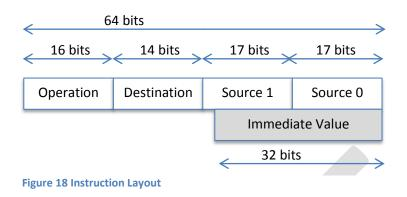
Each instruction section has special *fields* that modify the VP behavior in various ways. A very important field is the IMM field. The IMM field tells the VP whether it has to interpret the lowest 32 bits of the instruction as an immediate (literal) value, called IMMV, or as part of the register source sections. The IMM field also takes part in the addressing mode as discussed in section 3.6. Figure 19 illustrates how the VP interprets the instruction depending on the IMM bit.
