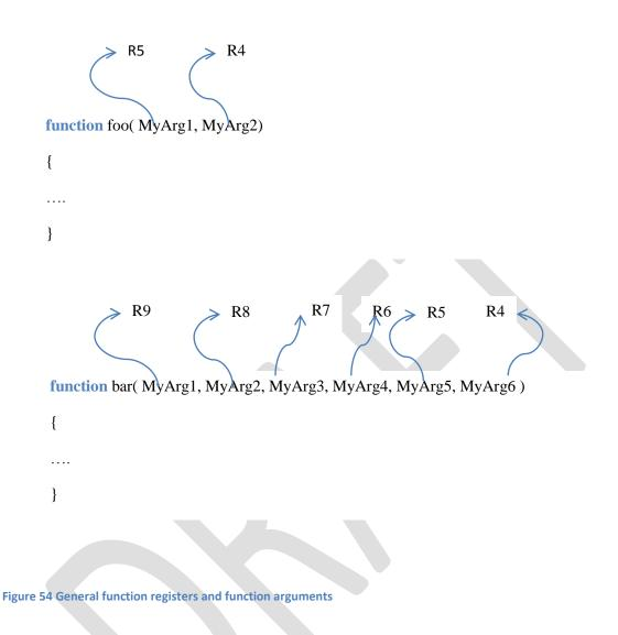
Note from the previous figure how the registers R4-R9 are assigned to the function arguments in reverse order.
