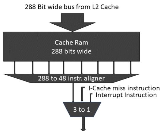
There are multiple copies of the L1 cache corresponding to the number of ways parallel of the core. Each copy may operate independently if SMT is enabled or in unison with other copies for a wider instruction fetch.
