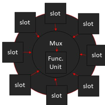
The instruction queue is circular with eight slots. Each slot feeds a multiplexor which in turn feeds a functional unit. Providing arguments to the functional unit is done under the vise of issue logic. Output from the functional unit is fed back to the same queue slot that issued to the functional unit. The queue slots are fed from the fetch buffers.
