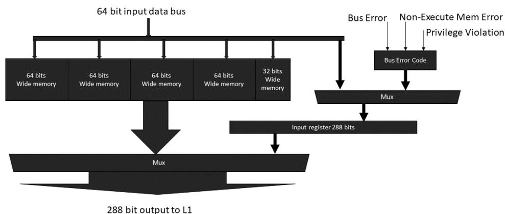
A cache load reads five words, four words for the cache line and a fifth word which is the first word of the next cache line, and stores four and a half words in the cache. The extra half-word is to accommodate 32 and 48 bit instructions that don't fit evenly into 256 bits and would overflow a 256 bit cache line. Cache line size is 36 bytes.
