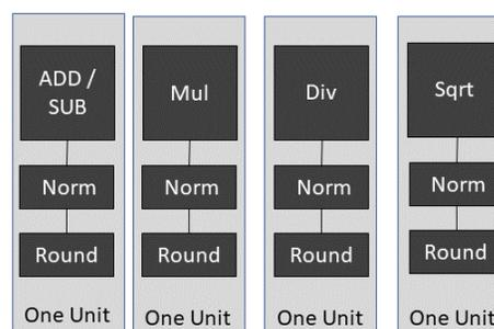
The current fp organization doesn't make good use of pipelining; one operation must complete before the next one can start. A faster fp organization allowing the use of pipelining is shown to the right. Other organizations with good performance are possible. The current unit focuses on small size.
