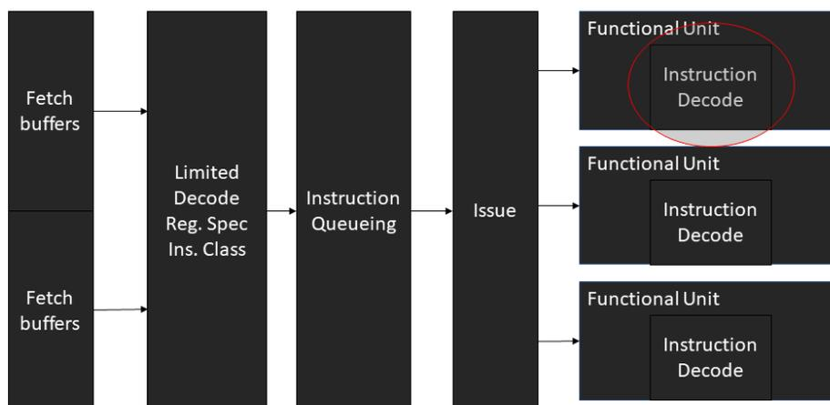
Limited decode takes place between fetch and queue. Between fetch and queue register specifications are decoded along with general instruction classes for the benefit of issue. A handful of additional signals (like sync) that control the overall operation of the core are also decoded. Much of the instruction decode is actually done in the functional unit. The instruction register is passed right through to the functional units in the core.
