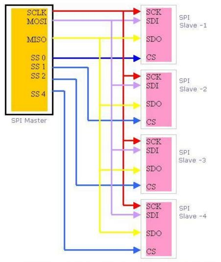
typical SPI-bus configuration with one SPI-master and multiple slaves/peripherals
