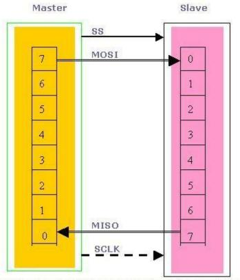
hardware setup for communication using two shift registers
