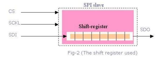
The slaves on the bus that has not been activated by the master using its slave select signal will disregard the input clock and MOSI signals from the master, and must not drive MISO. That means the master selects only one slave at a time.
