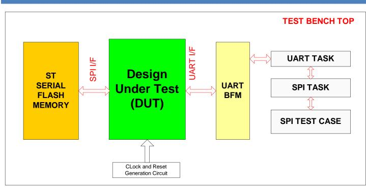
**UART Bus Functional Model (BFM):** This block manages the UART protocol format translation from 8bit data to serial format and vice-versa.
