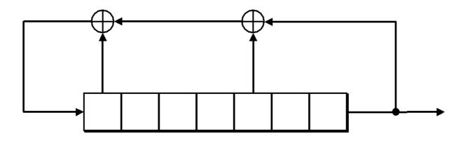
A **linear feedback shift register** (LFSR) is a shift register whose input bit is a linear function of its previous state.
