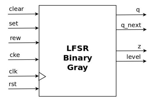
Top level module input and output signals
