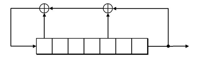
A **linear feedback shift register** (LFSR) is a shift register whose input bit is a linear function of its previous state.
