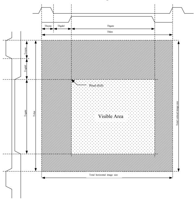
The video frame is composed of Tvlen video lines, each Thlen pixels long. The logical AND function of the horizontal gate and the vertical gate defines the visible area, the rest of the image is blanked.
