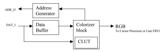
The Color Processor, together with the WISHBONE Master interface and the Line FIFO, handles the pixel color generation. The internal structure of the Color Processor, including parts of the WISHBONE Master interface, is shown in the figure above.
