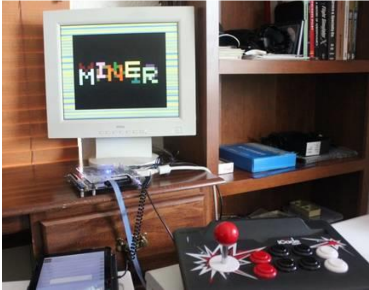
Image 3 : Sinclair ZX Spectrum on Altera DE1
