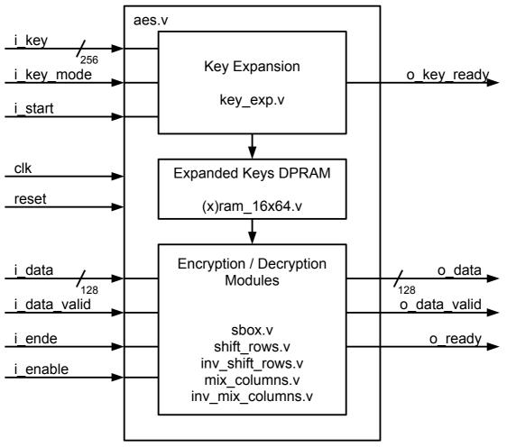
Figure 1: Simplified Core Block Diagram
