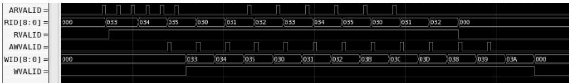
Illustration 15: Bus activity, two channels, 64 bit, buffer size 64 bytes, read and write outstanding
