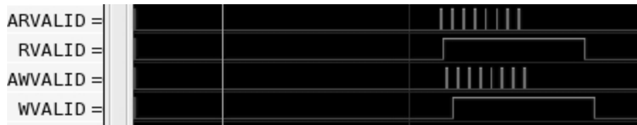
Illustration 13: Bus activity, single channel, 32 bit, buffer size 32 bytes, read and write outstanding
