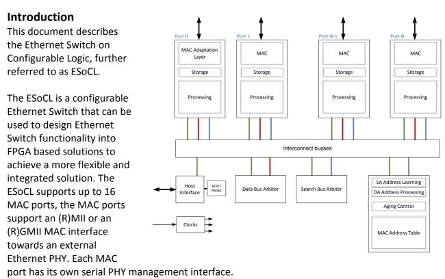
The ESoC is a VLAN capable Ethernet Switch. Untagged packets received by a port are tagged by the port default VLAN ID before they are processed. After switching an untagged packet to the destination port(s) the default tag is removed. Tagged packets can be re-tagged by the port default VLAN ID before or after they are processed further.
