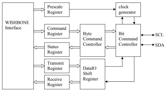
Fig. 5.1 Internal structure I2C Master Core
