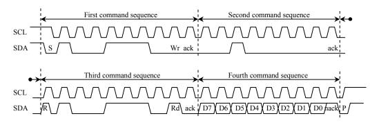
Please note that the time for the Interrupt Service Routine is not shown here. It is assumed that the ISR is much faster then the  $I^2C$  cycle time, and therefore not visible.
