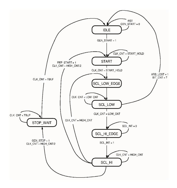
This machine will be used only in master mode to generate SCL pulses of desired frequency determined by PRESCALE register.
