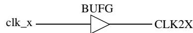
Figure 57. Spartan 3/e generation of CLK2X clock when VHDL generic clk2xen is zero
