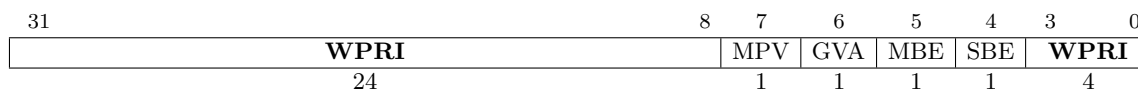
Figure 5.34: Additional machine status register ( mstatush ) for RV32 when the hypervisor extension is implemented. The format of mstatus is unchanged for RV32.
