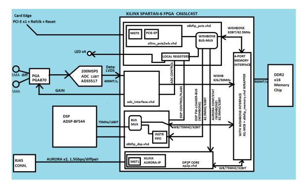
Prototype test board FPGA logic block diagram
