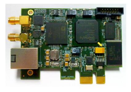
Prototype test board (S6BF\_BOARD without the FPGA-heat sink)
