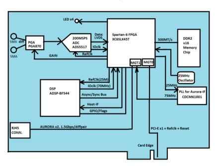
Prototype test board block diagram
