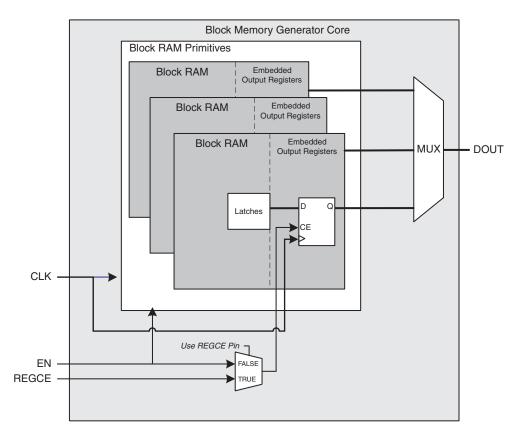
Figure 48: Spartan-6 or Spartan-3A DSP Block Memory Generated with Register Port [AIB] Output of Memory Primitives Enabled (No RST)
