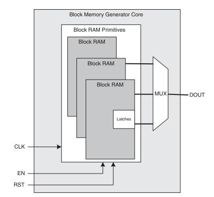
Figure 56: Spartan-3 Block Memory Generated with No Output Registers Enabled
