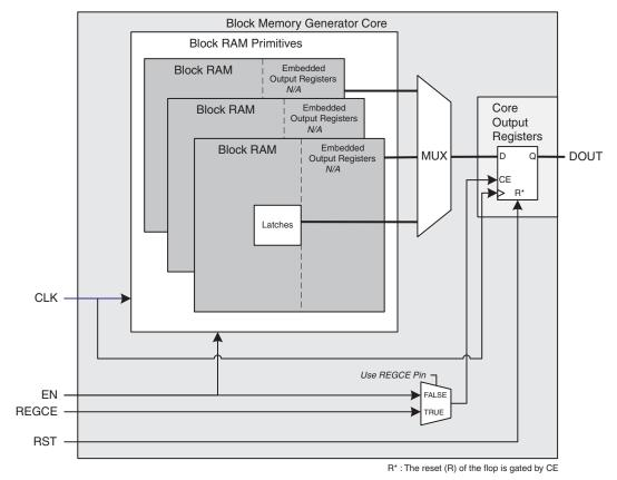
*Figure 45:* Virtex-6, Virtex-5, or Virtex-4 FPGA Block Memory Generated with Register Port [AIB] Output of Memory Core Enabled
