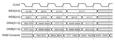
Figure 15: Write-write Collision Example
