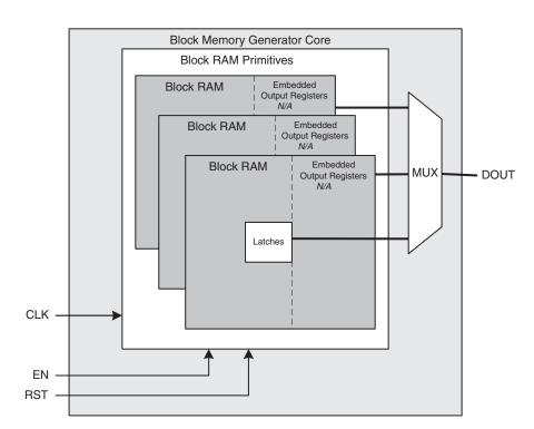
Figure 52: Spartan-6 or Spartan-3A DSP Block Memory Generated with No Output Port Registers Enabled
