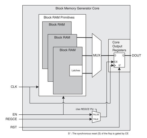
Figure 55: Spartan-3 Block Memory Generated with Register Port [AIB] Output of Memory Core Enabled
