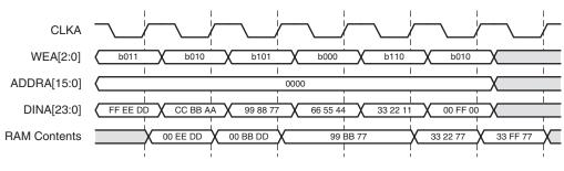
Figure 14: Byte-write Example
