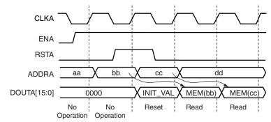
Figure 24: Standard Reset Behavior Similar to Previous Architectures
