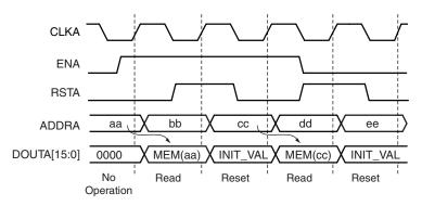
Figure 23: Reset Behavior When Reset Priority is Set to SR
