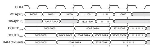
Figure 16: Write-read Collision Example
