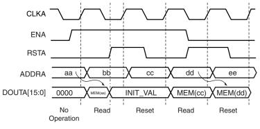
Figure 28: Asynchronous Reset
