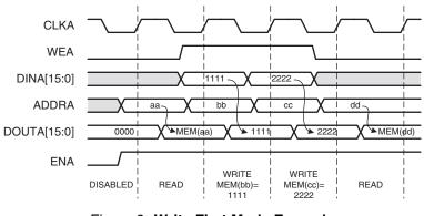
Figure 9: Write First Mode Example
