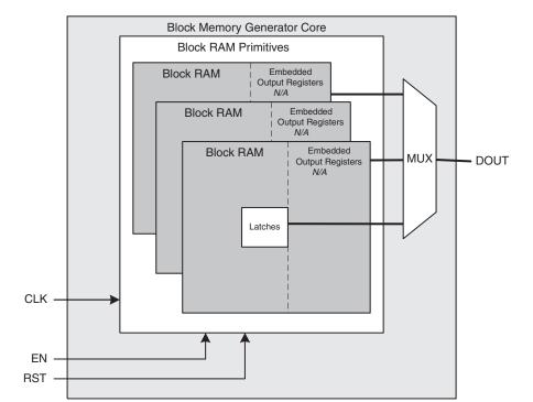
Figure 46: Virtex-6, Virtex-5 or Virtex-4 Block Memory Generated with No Output Registers Enabled
