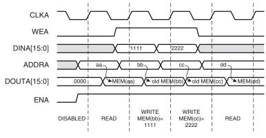
Figure 10: Read First Mode Example
