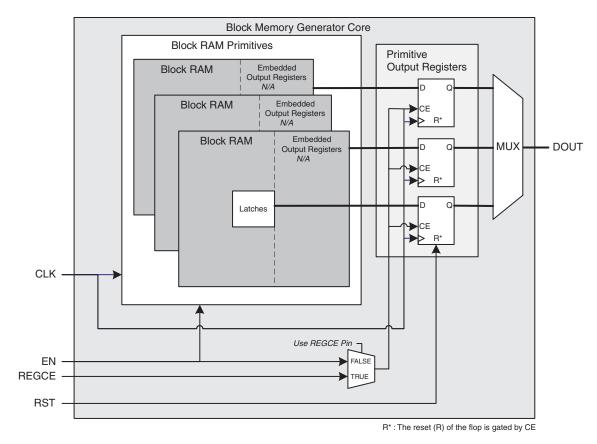
Figure 44: Virtex-4 Block Memory Generated with Register Output of Memory Primitives and Use RST[AIB] Pin Options Enabled
