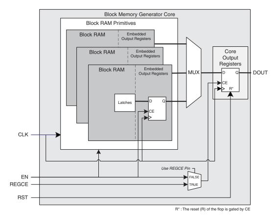
*Figure 39:* Virtex-6, Virtex-5, or Virtex-4 FPGA Block Memory Generated with Register Port [AIB] Output of Memory Primitives and Register Port [AIB] Output of Memory Core Enabled
