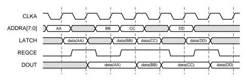
Figure 21: Flow Control Using REGCE
