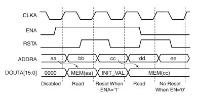
Figure 22: Reset Behavior When Reset Priority is Set to CE
