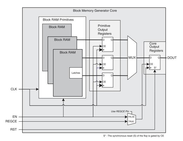
Figure 17: Spartan-3 Block Memory: Register Port [AIB] Outputs of Memory Primitives and Memory Core Options Enabled
