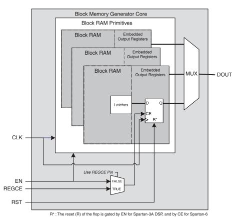
Figure 42: Virtex-5 FPGA Block Memory Generated with Register Port [AIB] Output of Memory Primitives Enabled
