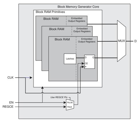
Figure 43: Virtex-4 Block Memory Generated with only Register Port [A | B] Output of Memory Primitives Enabled
