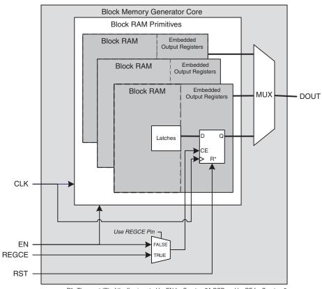
$\mathsf{R}^{\star}$  : The reset (R) of the flop is gated by EN for Spartan-3A DSP, and by CE for Spartan-6
