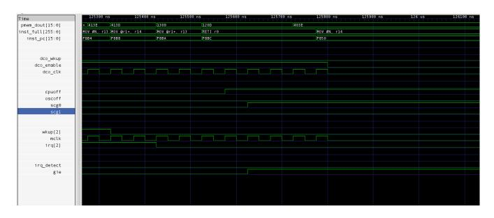
**Note:** the DCO oscillator is enabled until the BIS and RETI instruction are fully executed (i.e. until the CPU state machines reach their IDLE state).
