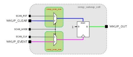
The basic idea here is simply to set the WKUP\_OUT signal with a rising edge on the WKUP\_EVENT port, and clear it when WKUP\_CLEAR is active (i.e. level sensitive clear).
