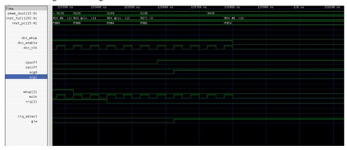
**Note:** the DCO oscillator is enabled until the BIS and RETI instruction are fully executed (i.e. until the CPU state machines reach their IDLE state).
