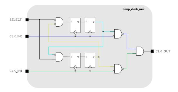
In order to make this implementation 100% bullet proof, the RTL could be modified by manually instantiating the NAND2 and AND2 cells directly from the target library (with the associated *don't touch* or *size only* attributes of course).
