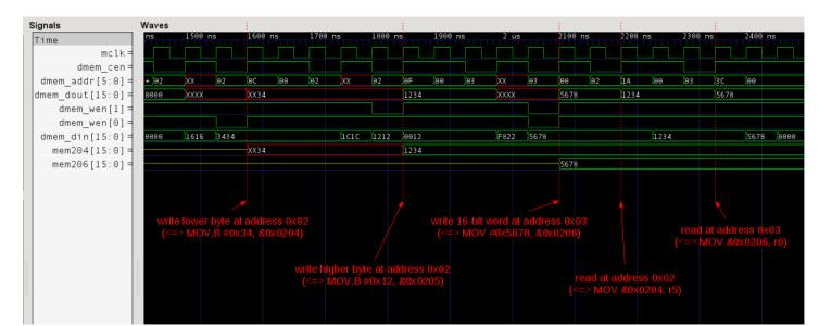
The following waveform illustrates some read/write access to the data memory:
