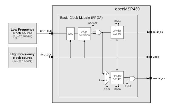
**Note**: CPUOFF doesn't switch MCLK off and will instead bring the CPU state machines in an IDLE state while MCLK will still be running.
