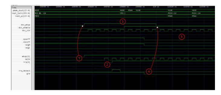
In order to wake-up the CPU from ANY low power mode, the system **MUST ALWAYS** go through the following chain of events (as illustrated in the previous waveform):
