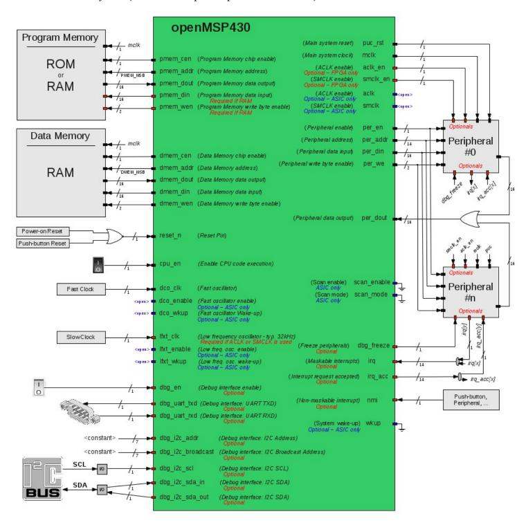
The full pinout of the core is summarized in the following table.
