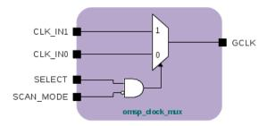
**Note:** if the LFXT clock domain is enabled, the *LFXT\_CLK* input port should also be connected to the scan clock when in scan mode.
