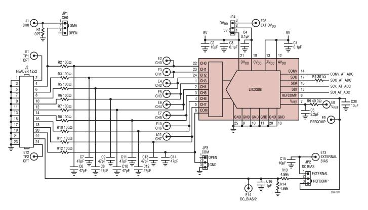
Figure 7f. Partial Demo Board Schematic
