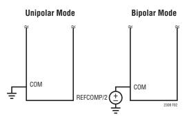
Figure 2. Driving COM in UNIPOLAR and BIPOLAR Modes
