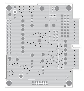
Figure 7d. Layer 3 Power Plane
