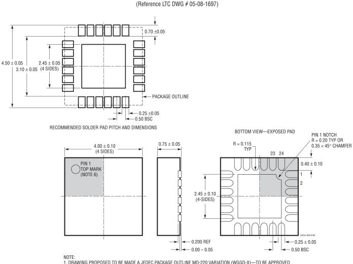
**UF Package** 24-Lead Plastic QFN (4mm × 4mm)
