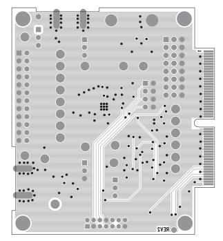
Figure 7e. Layer Back Solder Side
