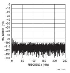
Figure 5. 1kHz Sine Wave 8192 Point FFT Plot
