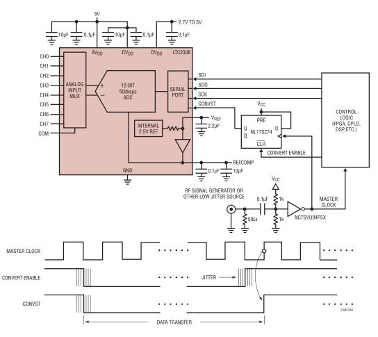
Clock Squaring/Level Shifting Circuit Allows Testing with RF Sine Generator, Convert Re-Timing Flip-Flop Preserves Low Jitter Clock Timing
