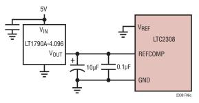
Figure 6c. Overdriving REFCOMP Using the LT1790A-4.096
