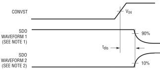
NOTE 1: WAVEFORM 1 IS FOR AN OUTPUT WITH INTERNAL CONDITIONS SUCH THAT THE OUTPUT IS HIGH UNLESS DISABLED BY THE OUTPUT CONTROL NOTE 2: WAVEFORM 2 IS FOR AN OUTPUT WITH INTERNAL CONDITIONS SUCH THAT THE OUTPUT IS LOW UNLESS DISABLED BY THE OUTPUT CONTROL 2200 TOUZ t<sub>WLCLK</sub> (SCK Low Time) t<sub>WHCLK</sub> (SCK High Time) t<sub>HD</sub> (Hold Time SDI After SCK↑) t<sub>SUDI</sub> (Setup Time SDI Stable Before SCK↑)
