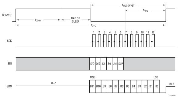
Figure 8. LTC2308 Timing with a Long CONVST Pulse
