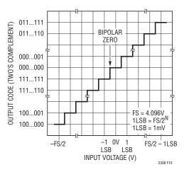
Figure 10. LTC2308 Bipolar Transfer Characteristics (2's Complement)
