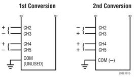
Figure 1b. Changing the MUX Assignment "On the Fly"
