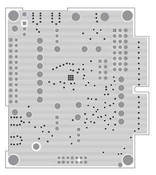
Figure 7c. Layer 2 Ground Plane
