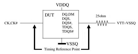
Figure 5.9.1 ODT Timing Reference Load
