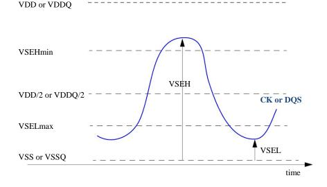
Figure 4.3.3 Single-ended requirement for differential signals.
