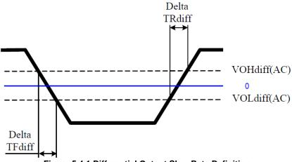
Figure 5.4.1 Differential Output Slew Rate Definition
