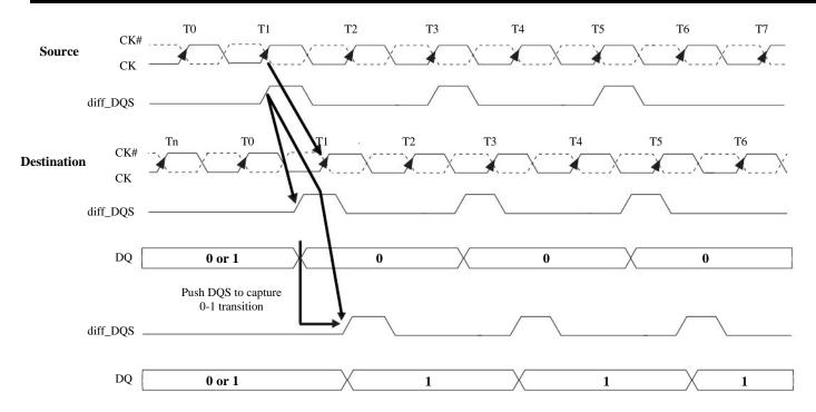
Figure 2.4.7 Write Leveling Concept
