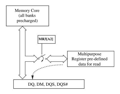
Figure 2.3.5.1 MPR Block Diagram
