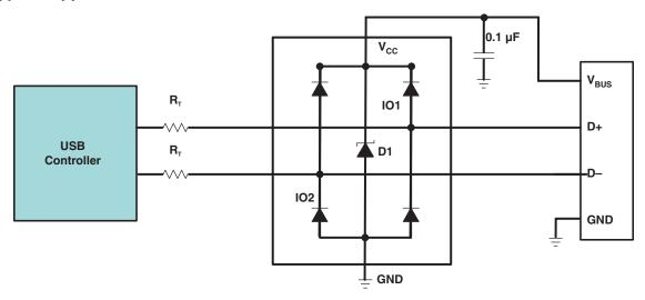
Figure 5. Typical USB Application Diagram
