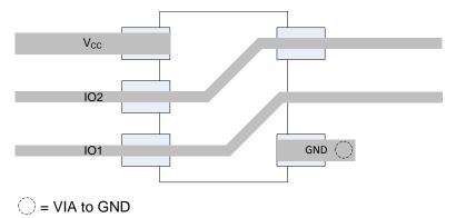
Figure 6. Routing with DRL Package
