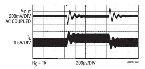
Figure 3a. Transient Response Shows Excessive Ringing
