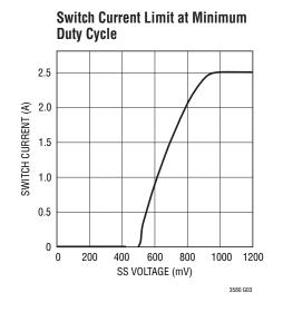
Switch Current Limit at Minimum Duty Cycle
