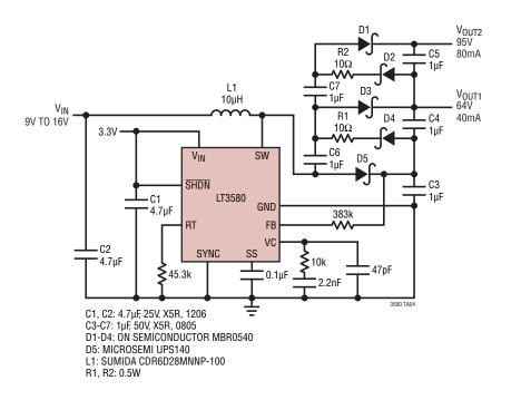
High Voltage Positive Power Supply Uses Tiny 5.8mm × 5.8mm × 3mm Transformer and Switches at 200kHz
