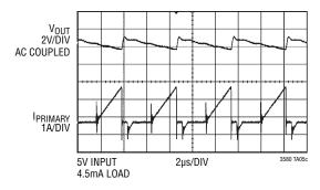
High Voltage Negative Power Supply Uses Tiny 5.8mm  $\times$  5.8mm  $\times$  3mm Transformer and Switches at 200kHz
