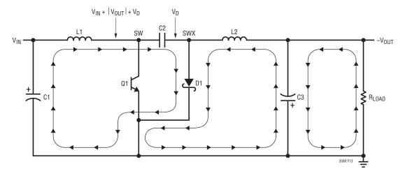
Figure 13. Switch-Off Phase of an Inverting Converter. L1 and L2 Currents Have Negative dI/dt
