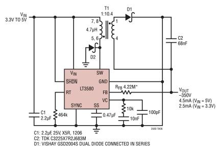
FOR ANY  $V_{OUT}$  BETWEEN –50V TO –350V, CHOOSE  $R_{FB}$  ACCORDING TO
