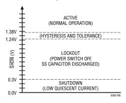
Figure 6. Chip States vs SHDN Voltage
