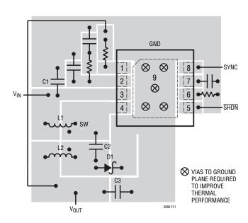
Figure 11. Suggested Component Placement for Inverting Topology (Both DFN and MSOP Packages. Not to Scale). Note Cut in Ground Copper at Diode's Cathode. Pin 9 (Exposed Pad) Must be Soldered Directly to Local Ground Plane for Adequate Thermal Performance. Multiple Vias to Additional Ground Planes Will Improve Thermal Performance
