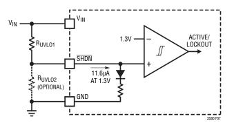
Figure 7. Configurable UVLO
