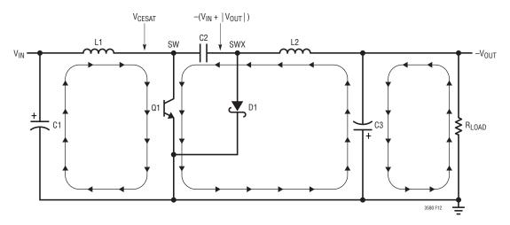
Figure 12. Switch-On Phase of an Inverting Converter. L1 and L2 Have Positive dl/dt
