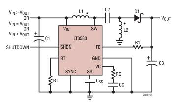
Figure 1. SEPIC Topology Allows for the Input to Span the Output Voltage. Coupled or Uncoupled Inductors Can Be Used. Follow Noted Phasing if Coupled
