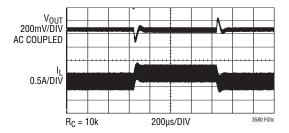
Figure 3c. Transient Response Is Well Damped
