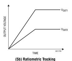
Figure 5. Two Different Modes of Output Voltage Tracking
