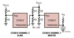
Figure 6a. Set-Up for Coincident Tracking
