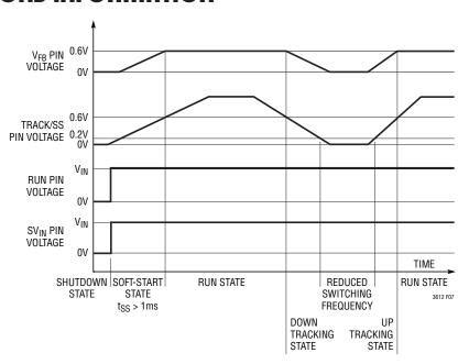
Figure 7. DDR Pin Not Tied to  $S_{VIN}$
