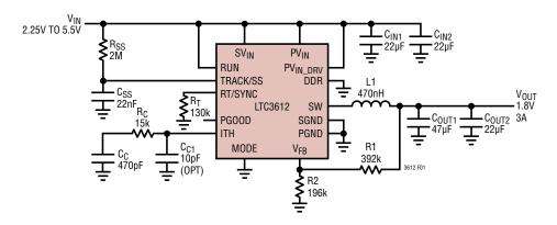
Figure 1. 1.8V, 3A Step-Down Regulator
