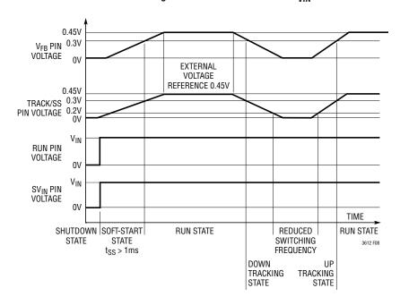
Figure 8. DDR Pin Tied to SV<sub>IN</sub>. Example DDR Application
