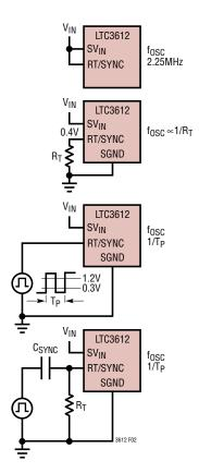
Figure 2. Setting the Switching Frequency
