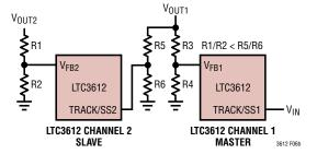
Figure 6b. Set-Up for Ratiometric Tracking
