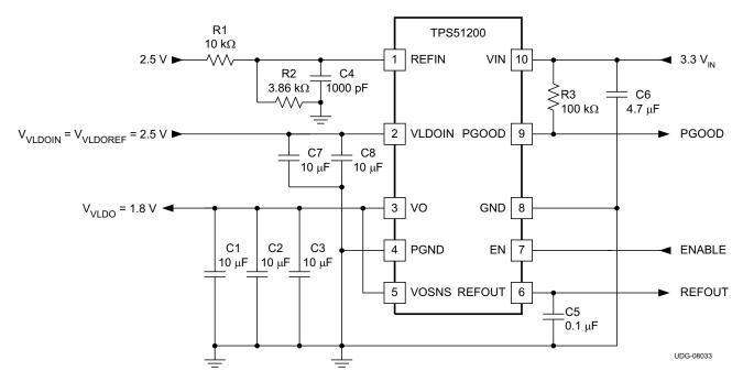
Figure 30. 3.3-V<sub>IN</sub>, LDO Configuration
