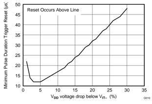
Figure 15. TPS3839 Transient Rejection
