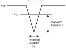
Figure 14. Voltage Transient Measurement
