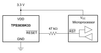
Figure 17. Connection to Bidirectional Reset Pin
