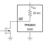
Figure 16. Using Logic-Level FET to Minimize Current Draw
