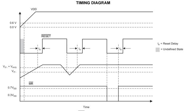
Figure 1.  $\overline{MR}$  and  $V_{DD}$  Reset Timing
