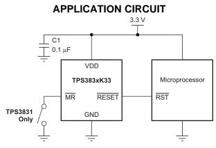
Figure 3. Typical Application Circuit
