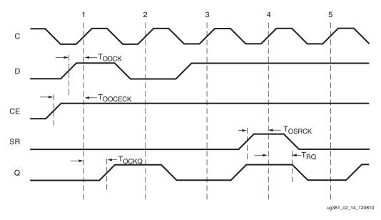
Figure 2-15: OLOGIC2 Output Register Timing Characteristics
