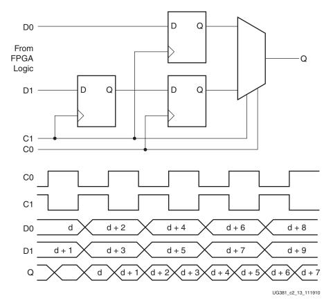
Figure 2-13: ODDR2 with DDR\_ALIGNMENT = C1
