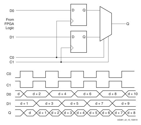
Figure 2-11: ODDR2 with DDR\_ALIGNMENT = NONE
