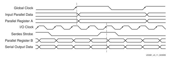
Figure 3-11: OSERDES2 Timing Diagram (4:1 Illustrated)
