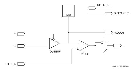
Figure 1-2: Basic IOB Diagram
