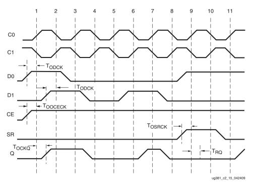
Figure 2-16: OLOGIC2 ODDR Register Timing Characteristics
