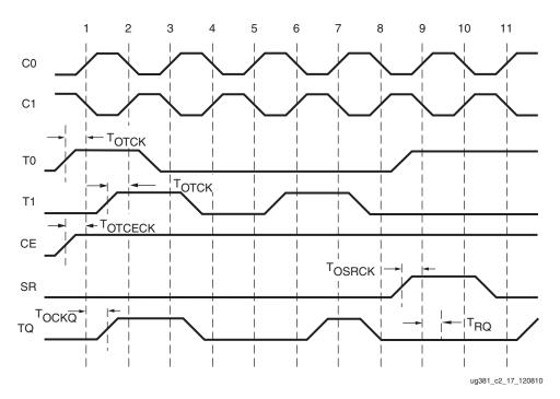
Figure 2-18 illustrates IOB DDR 3-state register timing. This example is shown using DDR ALIGNMENT = NONE.
