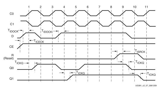
Figure 2-9: ILOGIC2 in IDDR2 Mode Timing Characteristics
