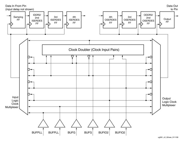
Figure 2-2: IOI Interface Logic Clocking Resources
