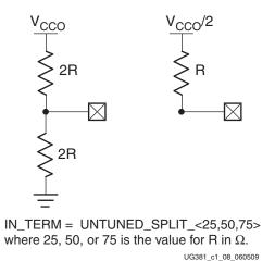
Figure 1-8: Input Termination for Split Termination
