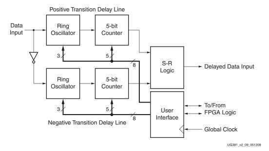
Figure 2-20: Using Two Delay Lines Per Delay Block
