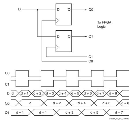
Figure 2-5: Input DDR when DDR\_ALIGNMENT = NONE
