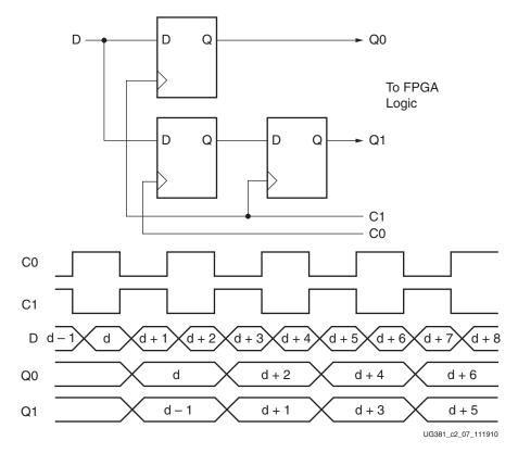
Figure 2-7: Input DDR When DDR\_ALIGNMENT = C1
