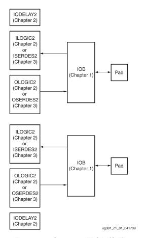
Figure 1-1: Spartan-6 FPGA I/O Tile
