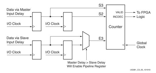
Figure 3-5: Phase Detector Operation
