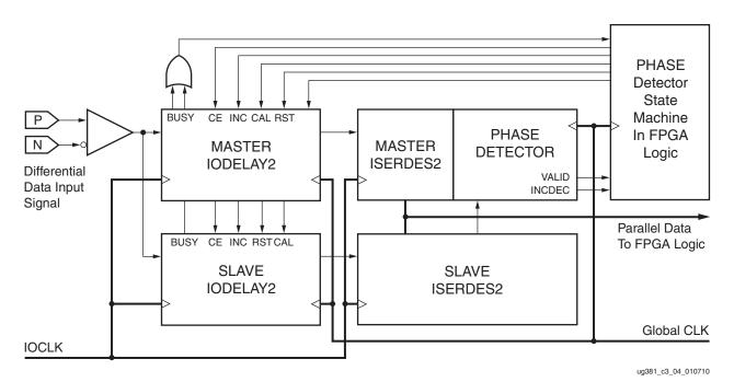
Figure 3-4: Differential Data-Phase Detector Topology Overview
