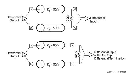
Figure 1-4: Differential Inputs and Outputs
