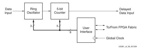
Figure 2-19: Delay Line Building Block
