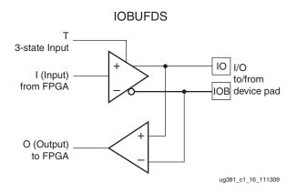
Figure 1-17: Differential Input/Output Buffer Primitive (IOBUFDS)
