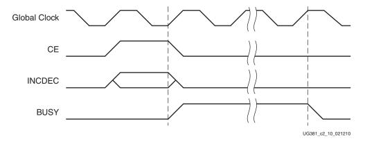
Figure 2-21: Delay Increment or Decrement Adjustment Timing
