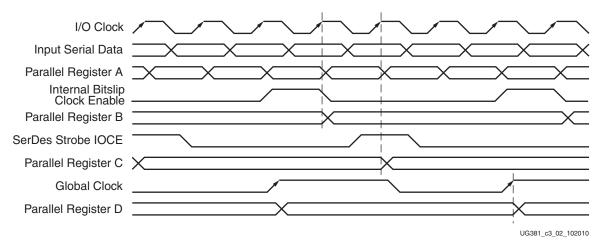
Figure 3-2: ISERDES2 Timing Diagram (4:1 Illustrated)
