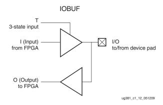
Figure 1-12: Input/Output Buffer (IOBUF) Primitive
