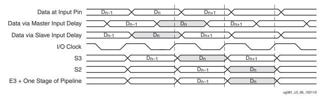
Figure 3-6: Phase Detector Internal Timing for Early Data Sampling–Check for S3 ≠ S2 and E3 = S3
