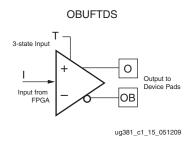
Figure 1-16: Differential 3-state Output Buffer Primitive (OBUFTDS)
