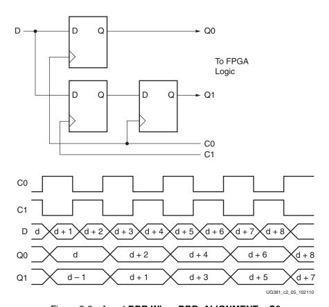
Figure 2-6: Input DDR When DDR\_ALIGNMENT = C0
