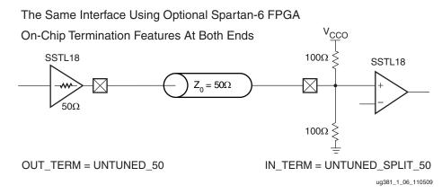
Figure 1-6: Unidirectional SSTL18 Interface Using On-Chip Termination
