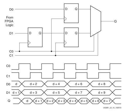
Figure 2-12: ODDR2 with DDR\_ALIGNMENT = C0
