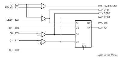
Figure 2-3: ILOGIC2 Block Diagram
