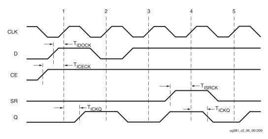
Figure 2-8: ILOGIC2 Input Register Timing Characteristics
