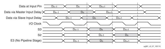
Figure 3-7: Phase Detector Internal Timing for Late Data Sampling—Check for S3 ≠ S2 and E3 = S3
