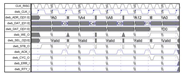
Figure 8. WISHBONE Block Read/Write Cycle
