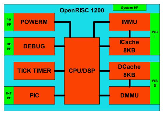
Figure 1. Core's Architecture
