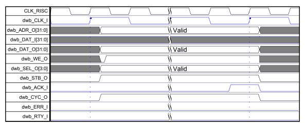
Figure 6. WISHBONE Write Cycle
