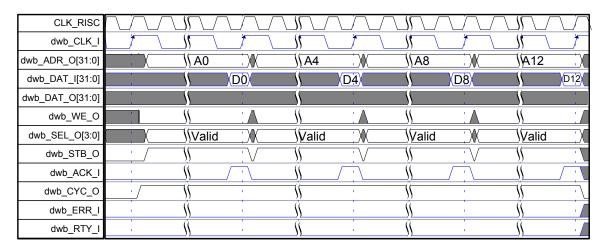
Figure 7. WISHBONE Block Read Cycle
