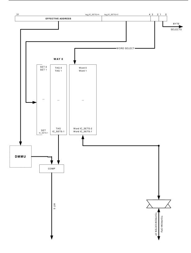
Each line contains four contiguous words from memory that are loaded from a four-word aligned boundary. As a result, cache lines are aligned with page boundaries.
