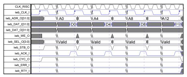
Figure 9. WISHBONE Block Read Cycle
