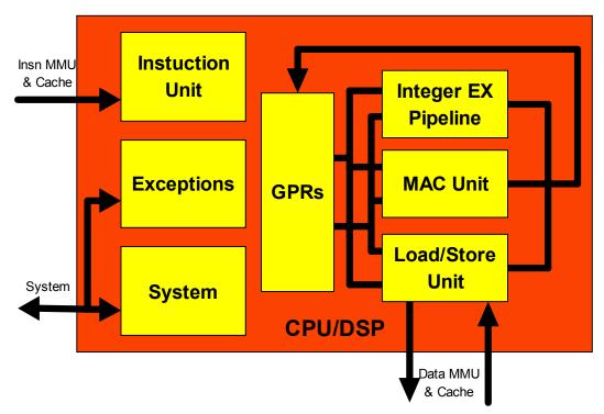
Figure 2. CPU/DSP Block Diagram
