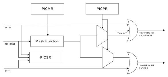
Table 5. Block Diagram of the Interrupt Controller
