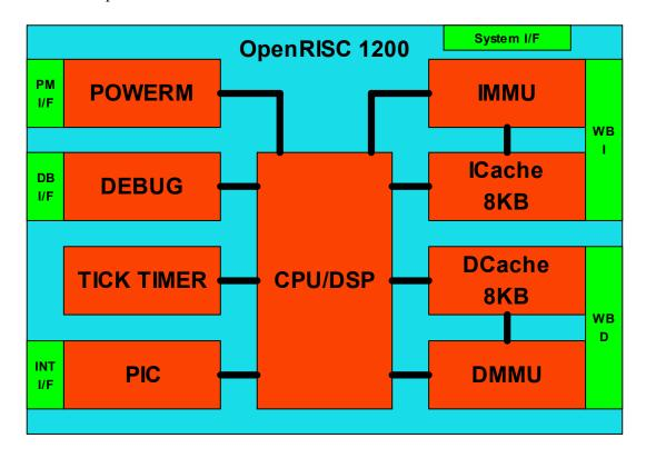
Figure 14. Core's Interfaces
