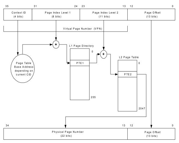
Figure 11. 32-bit Address Translation Mechanism using Two-Level Page Table
