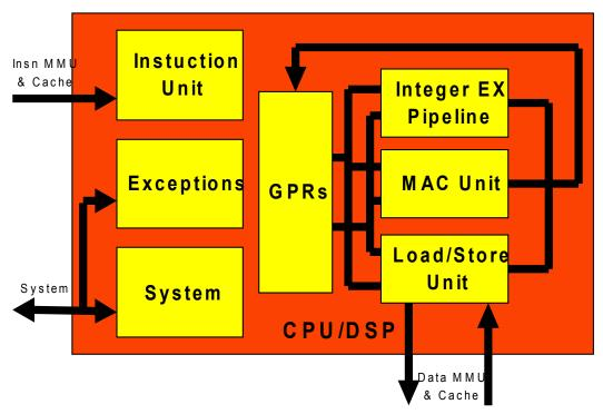
Figure 2. CPU/DSP Block Diagram
