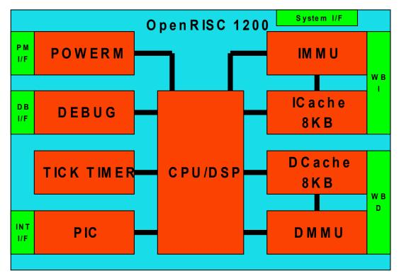
Figure 1. Core's Architecture
