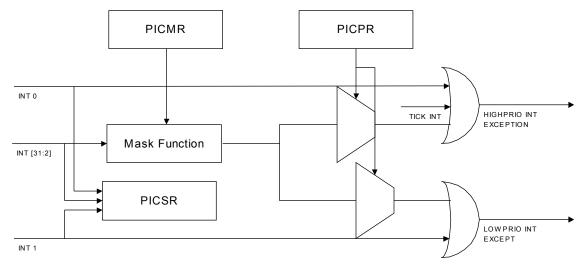
Table 5. Block Diagram of the Interrupt Controller
