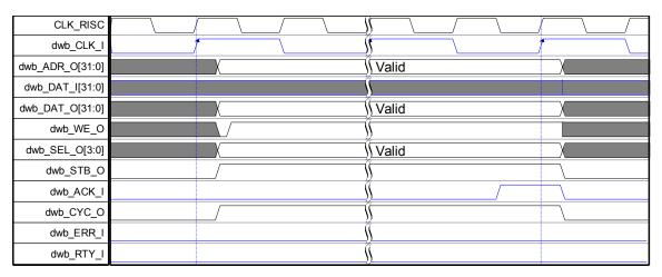
Figure 6. WISHBONE Write Cycle
