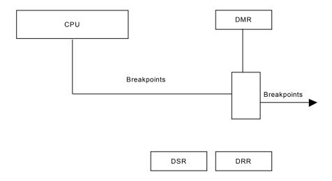
Figure 3. Block Diagram of Debug Unit
