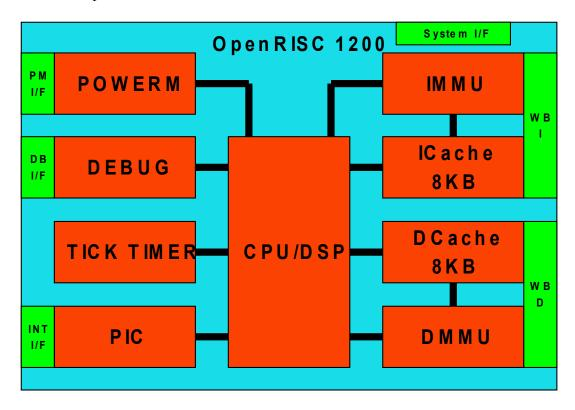
Figure 14. Core's Interfaces
