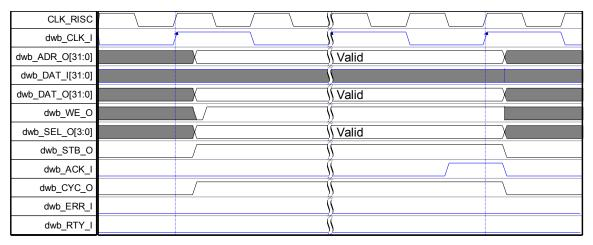
Figure 6. WISHBONE Write Cycle
