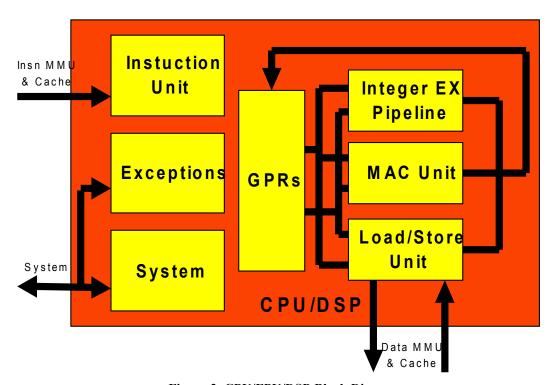
Figure 2. CPU/FPU/DSP Block Diagram
