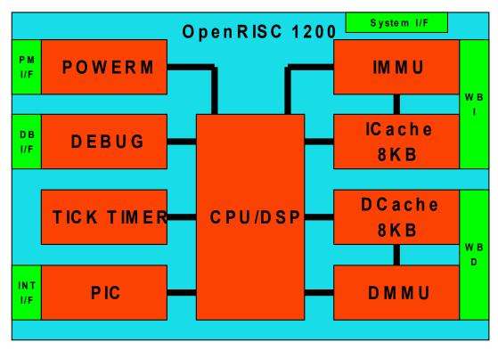
Figure 1. Core's Architecture
