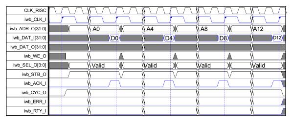
Figure 9. WISHBONE Block Read Cycle
