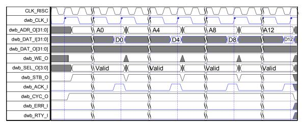
Figure 7. WISHBONE Block Read Cycle
