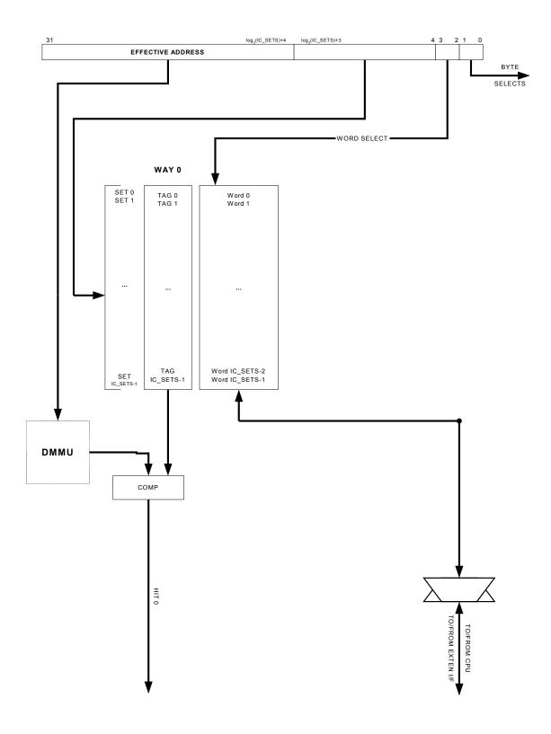
Each line contains four contiguous words from memory that are loaded from a line-size aligned boundary. As a result, cache lines are aligned with page boundaries.
