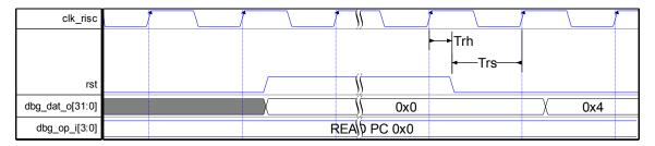
Figure 4. Power-Up and Reset Sequence
