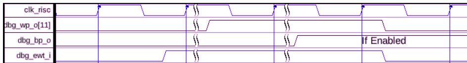
Figure 3.10: Assertion of External Watchpoint Trigger
